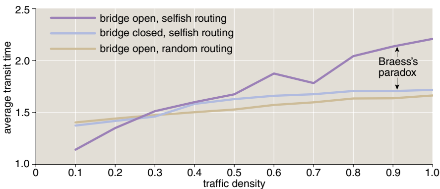
Transit time in the model network shows the cost of selfish routing, as well as the paradoxical effect that opening an extra road can slow everyone's trip. Except at very low traffic density, selfishly routed cars reach the destination faster when the midriver bridge is closed. Adopting a random routing strategy has an even greater benefit.
