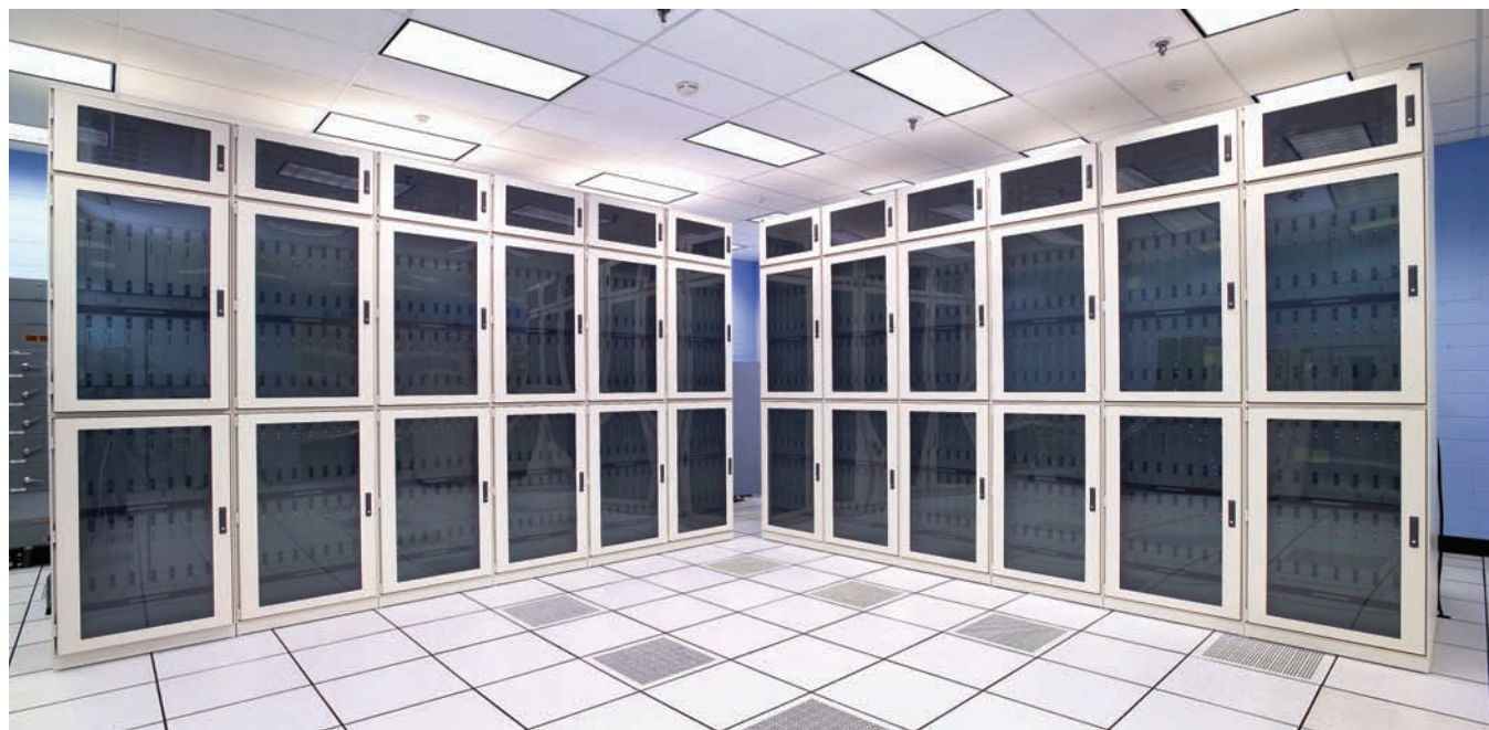
QCDOC, an abbreviation for QCD on a chip, is a series of computers designed specifically for lattice QCD calculations and dedicated more or less exclusively to that task. The glass-fronted cabinets seen here, at Brookhaven National Laboratory, hold two QCDOC machines, each with 12,288 processors; a third QCDOC is at the University of Edinburgh. (Photograph courtesy of Brookhaven National Laboratory.)
