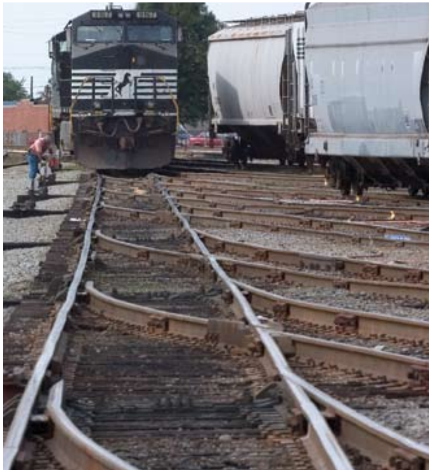
A railroad worker throws a switch lever in a small freight yard in Greensboro, North Carolina, where cars are put in order for delivery. Once the switch is set, the locomotive will couple to and pull out the line of cars farthest to the right. (Photograph by the author.)
