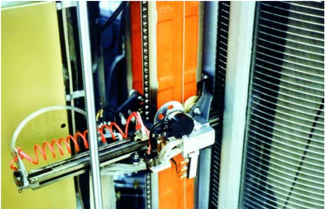
Figure 1. The first computer disk drive was built by IBM in 1956 as a component of a machine called RAMAC. Some of the 50 disk platters are visible at the right; each disk is two feet in diameter. The pneumatically controlled access mechanism, with a coiled orange cable, is in the center. (Photograph courtesy of Albert S. Hoagland of the Magnetic Disk Heritage Center in San Jose, http://www.mdhc.scu.edu .)
