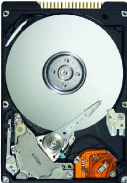
Figure 2. Modern disk drive has a glass platter two and a half inches in diameter, coated with an exotic sandwich of ferromagnetic alloys and ruthenium; the device is shown here at actual size. The single platter stores 15 gigabytes at a density of 25.7 gigabits per square inch. (At this density, the digitized photo of the drive would occupy less than two thousandths of a square inch of its own surface.) The drive is in the IBM Travelstar series.
