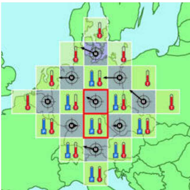
Figure 2. Data for Richardson's forecast included measurements of winds ( M ), barometric pressure ( P ) and temperature ( T ). Initial data were recorded in 25 squares, each 200 kilometers on a side, but conditions were forecast only for the two central squares outlined in red.
