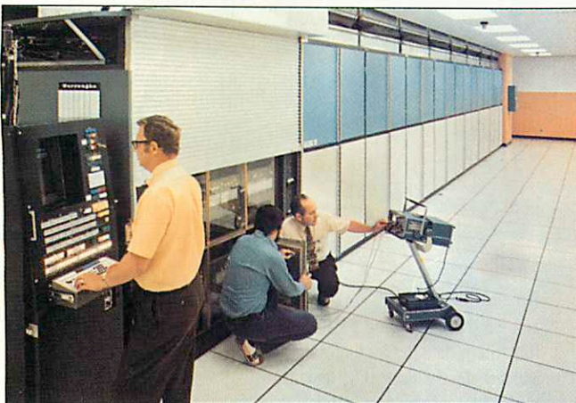
Illiac IV, an "array-processing" computer designed by the University of Illinois and Burroughs in the late 1960s. The computer consisted of 64 computers wired into an 8-by-8 matrix. Computations were performed in parallel.
