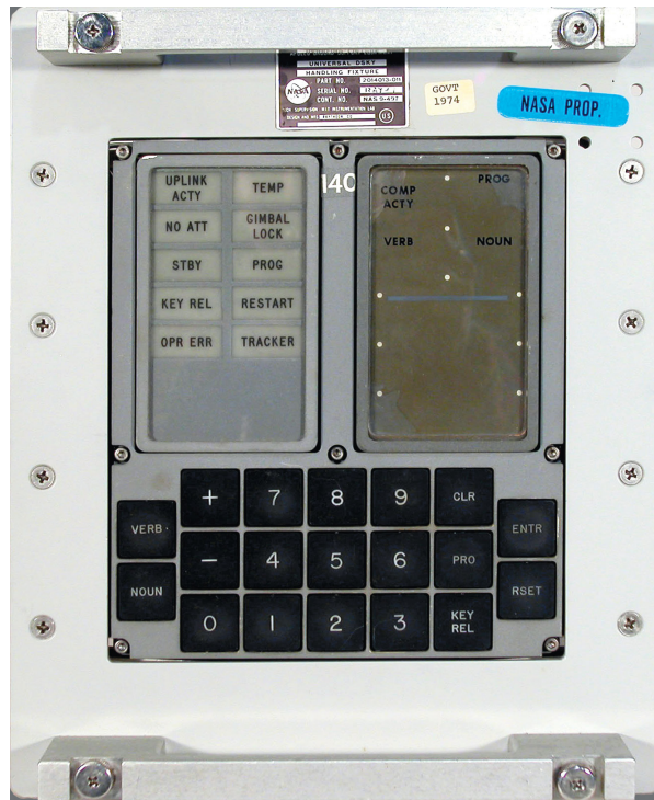
The AGCs in the command module and the lunar module were accessed by the astronauts through a "display keyboard" (DSKY) mounted in the module's control panel. Astronauts specified actions by entering a program, a verb, and a noun, all represented by two-digit numbers. The DSKY shown here is from the Smithsonian Air and Space Museum and never flew on an Apollo mission.
